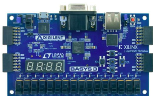
BASYS 3 FPGA board used for this experiment.
